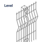
Use top hole of each set of three at the top and bottom
